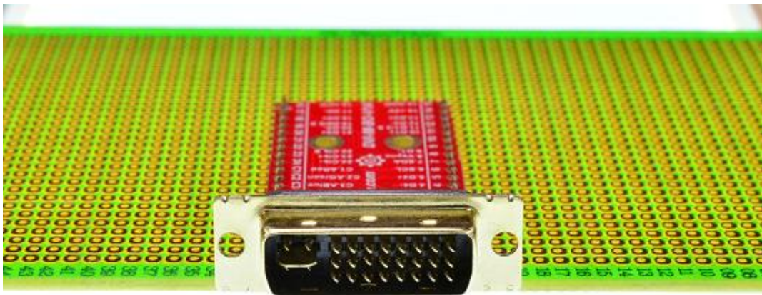
Figure 4: Solid Mounting on prototype PCB
