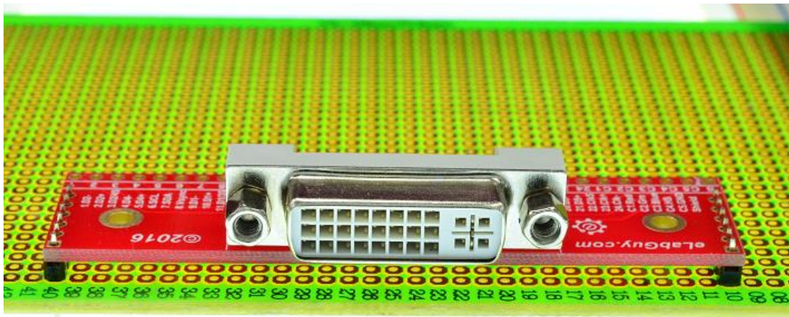
Figure 4: Solid Mounting on prototype PCB
