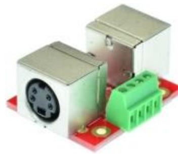
Figure 4: mDIN4-F-F-V1A with terminal blocks
