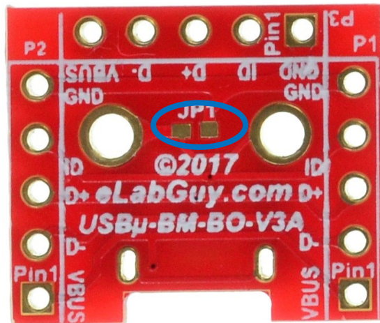
Figure 4: Optional Jumper connects Shield to GND
