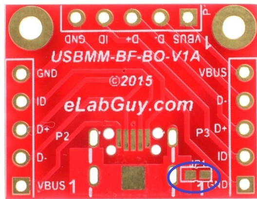
Figure 4: Optional Jumper connects Shield to GND
