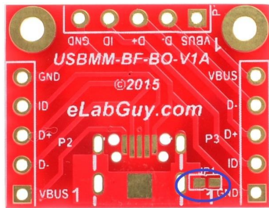
Figure 4: Optional Jumper connects Shield to GND
