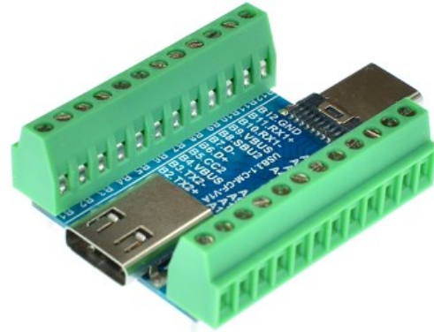
Figure 4: USB3.1-CM-CF-V1A with terminal blocks
