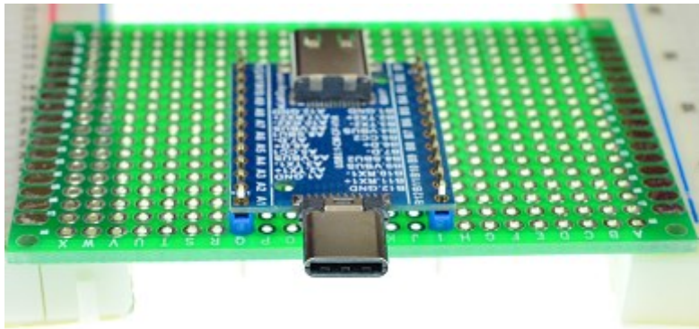
Figure 5: Solid Mounting on prototype PCB
