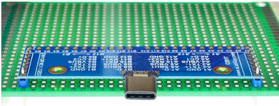
Figure 5: Solid Mounting on prototype PCB
