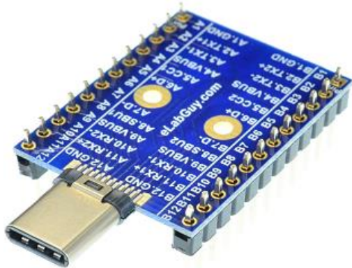
Figure 3: USB3.1-CM-BO-V2A with headers
