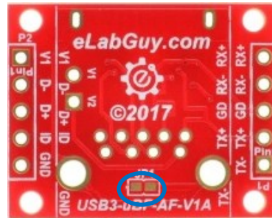
Figure 6: PCB back with optional Jumper connects Shield to GND
