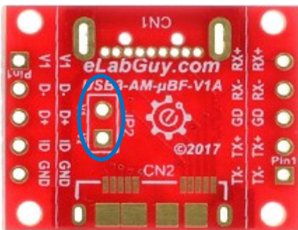
Figure 5: PCB front with open circuit on VCC pin in series
