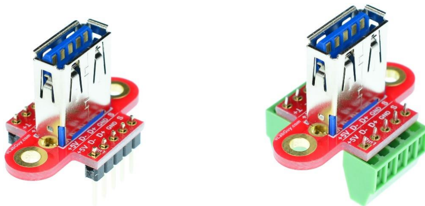
Figure 3: USB3-AF-BO-V1AV Various connections
