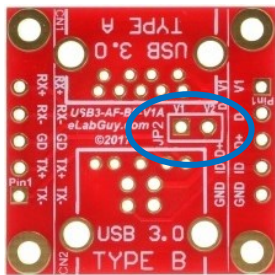
Figure 5: PCB front with open circuit on VCC pin in series
