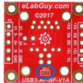
Figure 6: PCB back with optional Jumper connects Shield to GND
