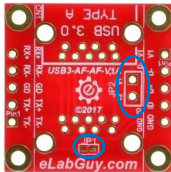
Figure 5: PCB back with optional Jumper connects Shield to GND and open circuit on VCC pin in series
