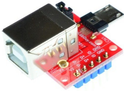
Figure 3: USB-uBM-BF-V1A with headers
