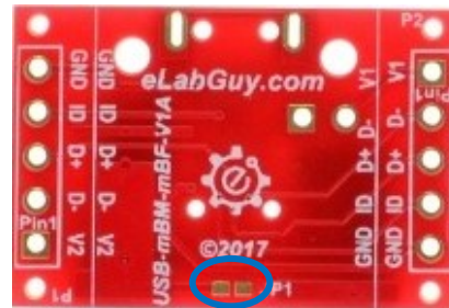
Figure 6: PCB back with optional Jumper connects Shield to GND
