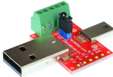
Figure 4: USB-mBM-AM-V1A with terminal blocks
