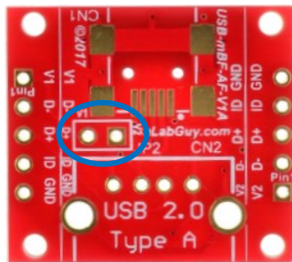
Figure 5: PCB front with open circuit on VCC pin in series
