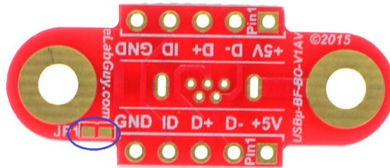
Figure 4: Optional Jumper connects Shield to GND
