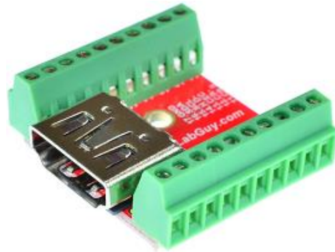
Figure 4: HDMI-AF-BO-V2A with terminal blocks
