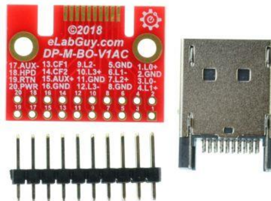
Figure 1: Parts inside the kit (Note: the module is not assembled, user can decide which connector to use on the module.)
