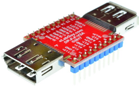
Figure 3: DP-F-F-V2A with headers
