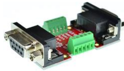
Figure 4: D9-F-F-V1A with terminal blocks
