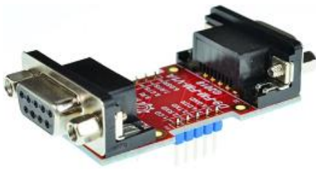
Figure 3: D9-F-F-V1A with headers
