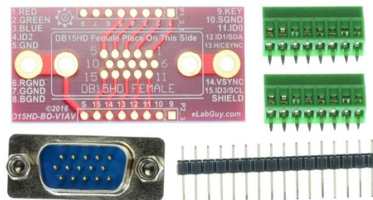
Figure 1: Parts inside the kit (Note: the module is not assembled, user can decide which connection to use on the module.)
