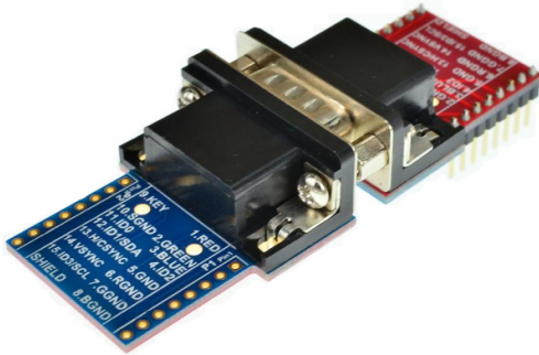
Figure 5: Solid Male to Female connection with the 4-40UNC diameter 8.3mm long screws
