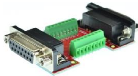
Figure 4: D15-M-M-V1A with terminal blocks
