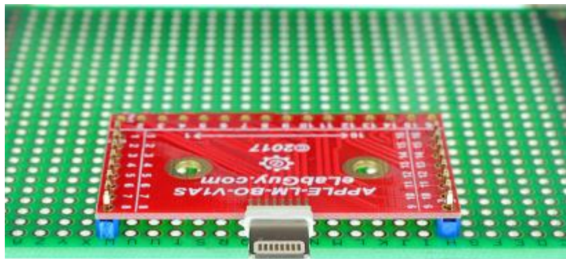
Figure 5: Solid Mounting on prototype PCB
