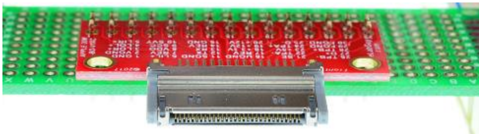
Figure 4: Solid Mounting on prototype PCB
