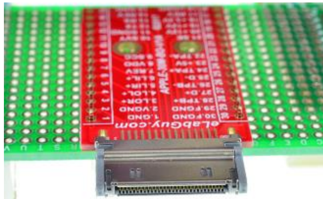
Figure 4: Solid Mounting on prototype PCB
